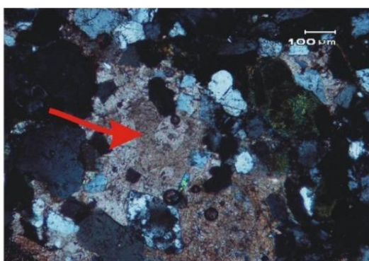
Fig. 7.6: Photomicrograph depicting complete dissolution of framework grains by carbonate cement
