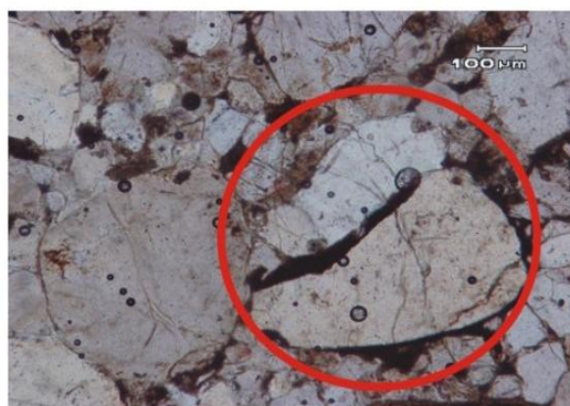
Fig. 7.3: Photomicrograph showing iron oxide cementation sandwiched between two grains (XPL)
