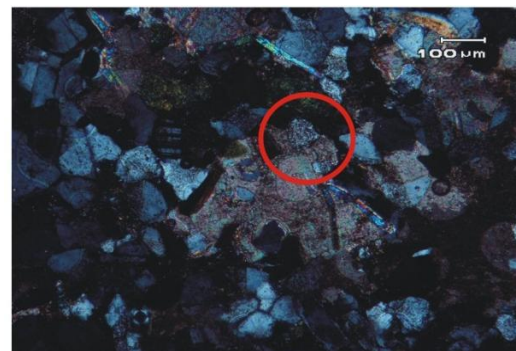
Fig. 4.16: Photomicrograph showing volcanic lithic fragment in central part of Kussak formation
