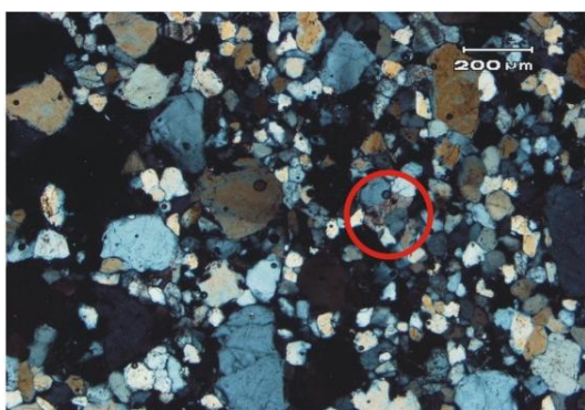
Fig. 7.7: Photomicrograph depicting partial dissolution of framework grains by carbonate cement
