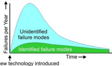
Figure 11. Typical failure trend for a new technology [14].
