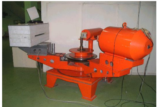
Fig. 4: PARR-1 double-axis diffractometer installed at beamtube 4.
