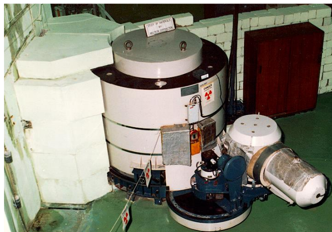
Fig. 3: Triple-axis diffractometer at beamtube 3, PARR-1.
