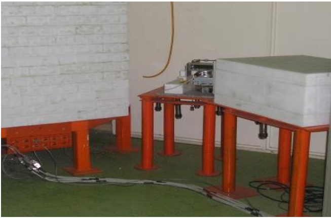
Fig. 5: Small angle neutron scattering instrument installed at beam tube 5, PARR-1.
