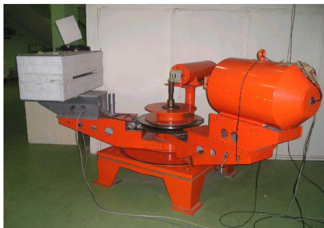
Fig. 4: PARR-1 double-axis diffractometer installed at beamtube 4.
