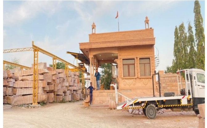
Fig. 2: Use of Sandstone as building materials – from quarried raw material i.e., slabs of sandstone (left side) to finished building of sandstone (right side).
