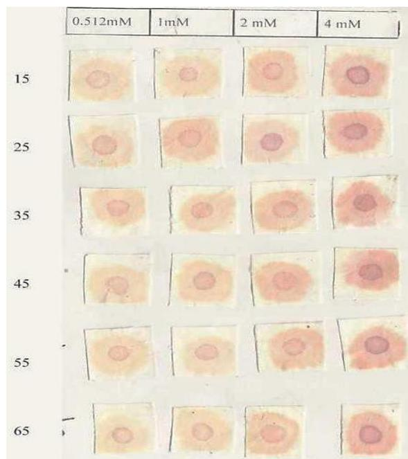
Fig. 7: Effect of temperature on bioactive paper platform 15-65 temperature in °C and from 0.512-4mM is substrate concentration
