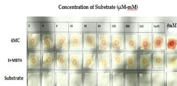
Fig. 4: Detection limit of bioactive paper platform
