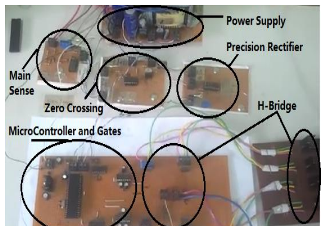
Fig. 9: Hardware of the proposed system.
