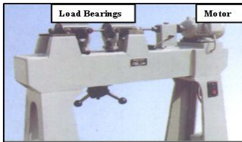
Fig. 2: Rotary bending fatigue testing
