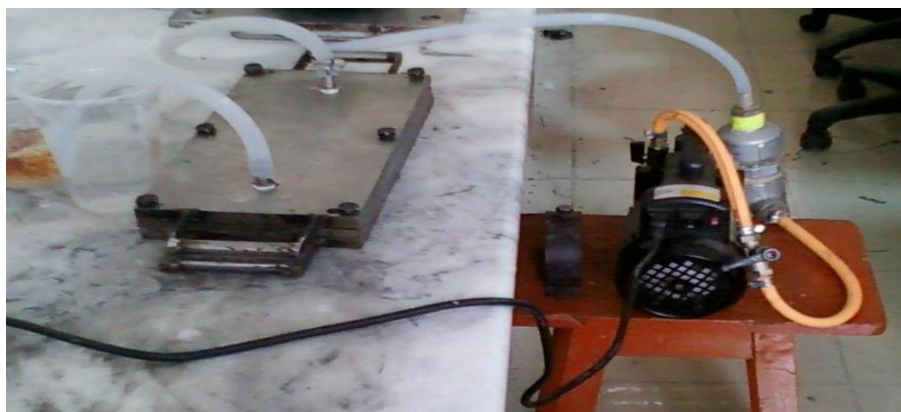
Figure 3. VARTM setup for dog bone mold.
