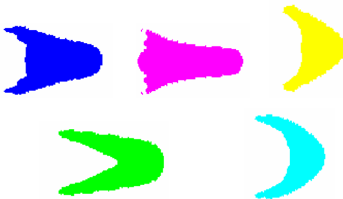
Figure 3: EFPs for mild steel, copper, tantalum, aluminum and armco Iron at stable velocity.
