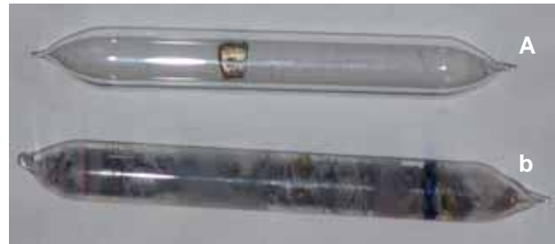
Figure-2. Alloy ingot encapsulated in the quartz tube back filled with argon gas.(A) before heat treatment (B) after heat treatment
