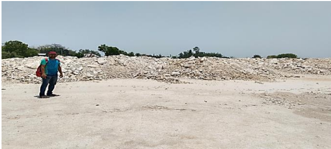
Fig. 3: Mined Clay locally stored in the dump yard, immediately after the mining and later on transported the raw clay to the factory for further processes.
