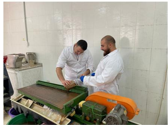
Fig. 4: Wilfley shaking table unit used in the experimental studies and the sketch showing the light, middling and heavy fractions (left) collecting points during beneficiation studies of heavy mineral sand.
