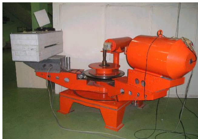
Fig. 4: PARR-1 double-axis diffractometer installed at beamtube 4.
