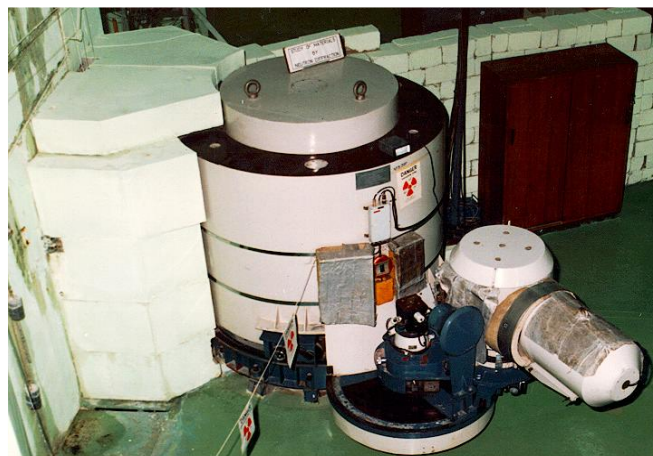
Fig. 3: Triple-axis diffractometer at beamtube 3, PARR-1.
